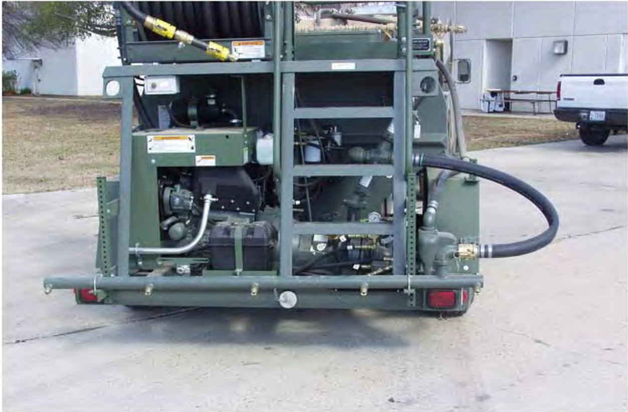
Photo 24. Distribution bar on rear of HydroSeeder
