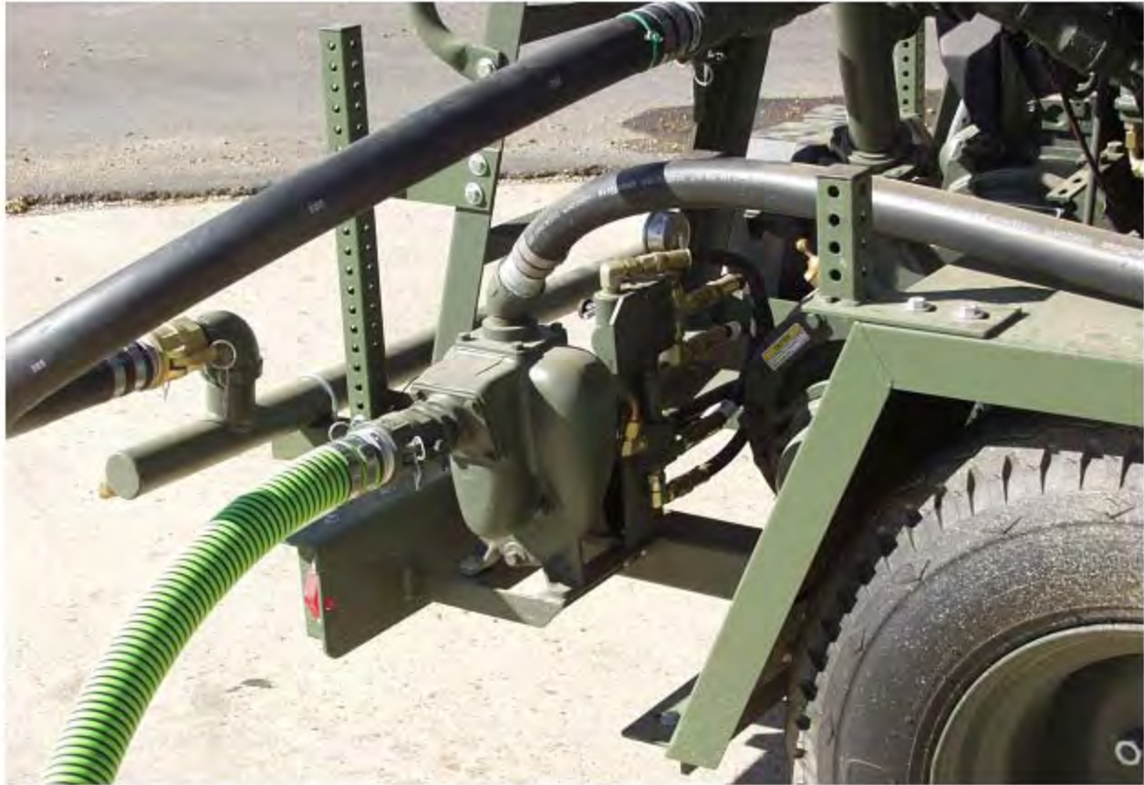
Photo 16. Filling HydroSeeder from storage container using onboard hydrostatic pump
