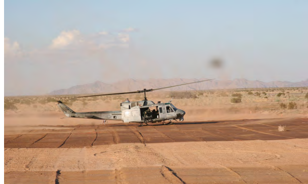
Photo 4. UH-1 landing on helipad treated with synthetic fluid
