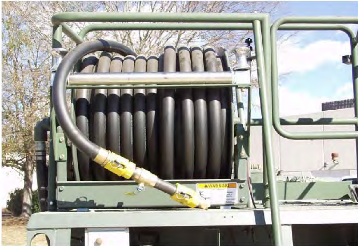
Photo 20. 200-ft hose with electric reel for multiple-use palliative distribution
