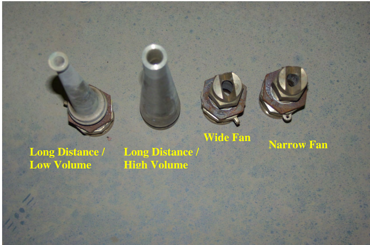
Photo 23. Spray nozzles for various spray patterns.
